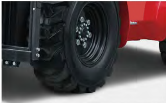
Large size deep pattern off-road vacuum tire with excellent off-road capability and shock absorption performance.
