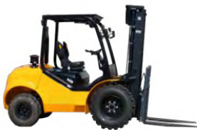
2WD SERIES 2.5T 3m Duplex Mast, Pneumatic Tyres FD25T FG30T FG35T
