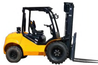
2WD SERIES 3.5T 3m Duplex Mast, Pneumatic Tyres FD25T FG30T FG35T
