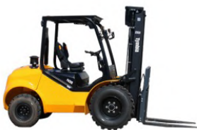
4WD SERIES 2.5T 3m Duplex Mast, Pneumatic Tyres
